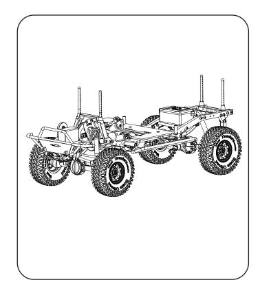
**Step 3.** Install the body on the chassis.
